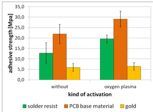
Fig. 1: Diagram of adhesive strength of EMC to different base materials of the PCB, untreated surfaces in comparison to O<sub>2</sub>-plasma activated surfaces.
