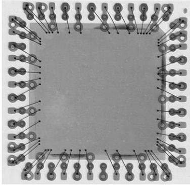
Fig. 3: X-ray radiography of a packaged QFN-FlexPac to determine possible failures of gold bond wires due to mass flow during molding.
