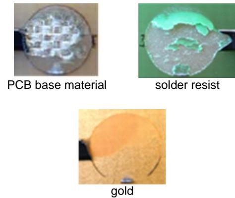
Fig. 2: Breakage areas of EMC on different base materials after shear tests of adhesion testing. Cohesion breakage could be observed for PCB base material and solder resist. Adhesion breakage was observed for the gold surface.
