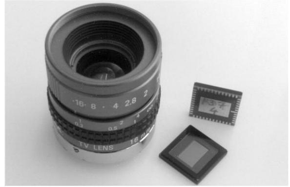
Fig. 8: Demo image using the image sensor packaged by the FlexPac process.
