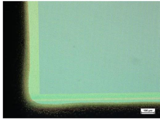
Fig. 6: Sealing edge of the ETFE foil at the sensor area. The soft seal of the ETFE foil in combination with precise alignment leads to well defined clearances.
