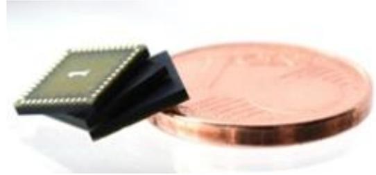
Fig. 4: QFN-FlexPac. Design rules and process parameters were optimized to qualify the method for general packaging.
